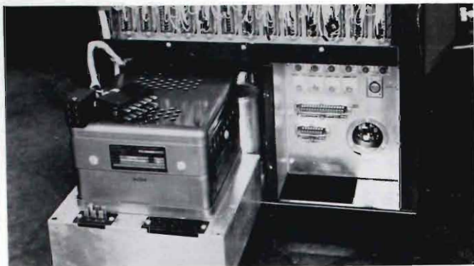
FIG. 9. Power deck of TR-3. At right is connector panel. At left is power supply.
