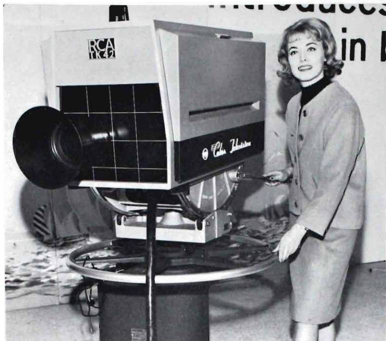
EXPERIMENTAL MODEL (1962). First 4-tube Color Camera to be shown anywhere was this experimental model of the RCA TK-42 which was exhibited at the 1962 NAB. Broadcasters comments were solicited and were incorporated in following models.
