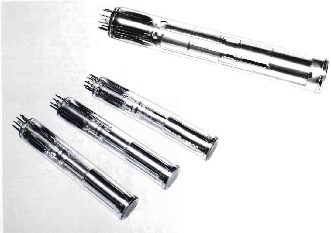
FIG. 18. Vidicon pickup tubes, 1½-inch monochrome type and three 1-inch color types, are all electrostatically focused, greatly reducing amount of heat usually dissipated in camera head.
