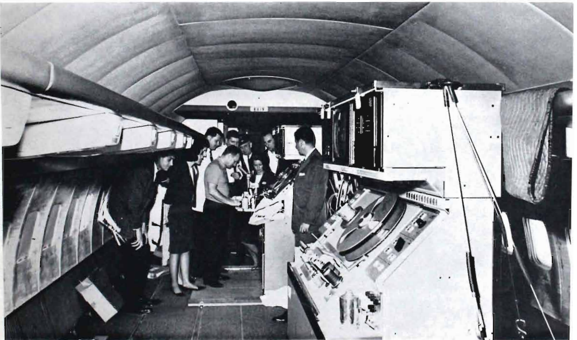
Seats were removed from the TWA Starstream to make room for the tape machines.
